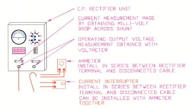
2) a current interrupter to cycle the output "Off" & "On"
