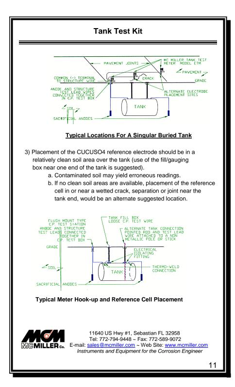
The test meter is connected so that the positive (+) terminal is connected to the CUCUSO4 electrode and the negative/common ( -) terminal is connected to the tank structure being tested.
