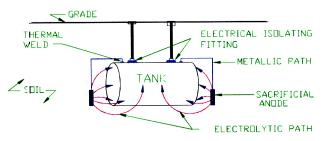
**Typical Galvanic Anode Installation**
