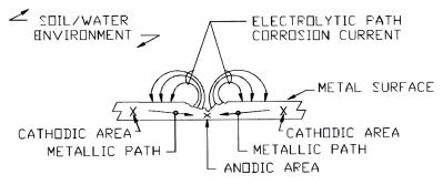
The Corrosion Process On a Steel Surface Exposed to a Corrosive Soil/Water Environment
